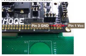
Connect pins 1 and 3 from the DEMO board to pins 1 and 3 respectively and insert the whole connector.
