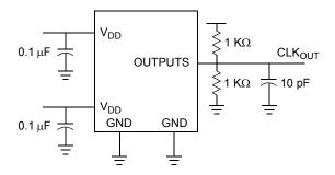
Test Circuit for t<sub>8</sub>, Output slew rate on -1H, -5 device
