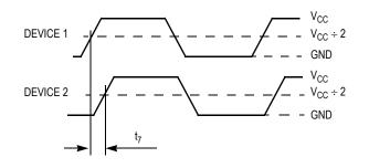
Figure 4. Device-to-Device Skew
