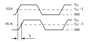
Figure 2. Static Phase Offset Test Reference
