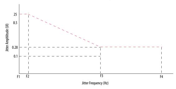
LVDS Soft-CDR/DPA Sinusoidal Jitter Tolerance Specification
