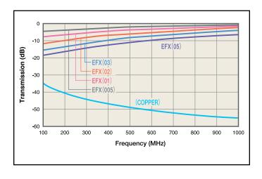
EFX - Attenuation of coupling noise
