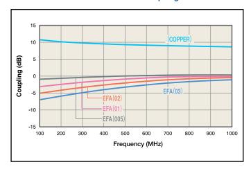
EFH - Attenuation of transmission noise
