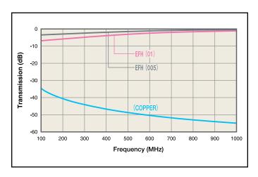
EFH - Attenuation of coupling noise
