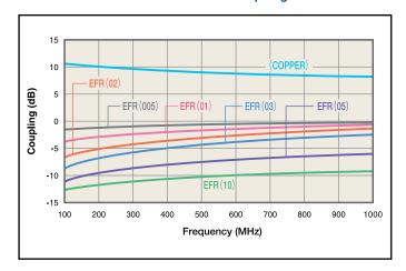
EFX - Attenuation of transmission noise
