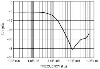
Figure 2. Insertion Loss Characteristics on Data Lines
