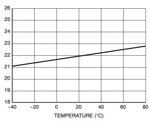
Figure 5. Typical Resistance over Temperature for  $R_1$  and  $R_2$
