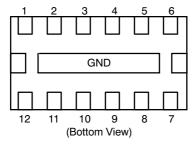
**Figure 1. Pin Connections**
