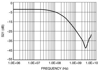
Figure 3. Insertion Loss Characteristics on USB Lines
