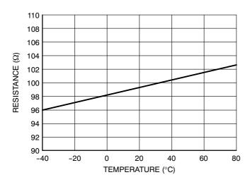
Figure 6. Typical Resistance over Temperature for  $R_3 - R_6$
