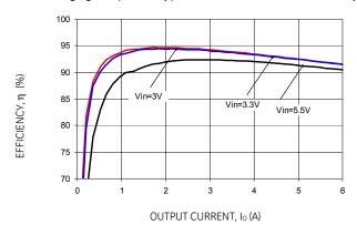
Figure 19. Converter Efficiency versus Output Current.
