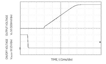
Figure 17. Typical Start-up Using On/Off Voltage ( $I_0 = I_{o,max}$ ).
