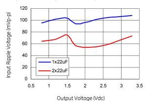
Figure 34. Input ripple voltage for various output voltages with 1x22  $\mu F$  or 2x22  $\mu F$  ceramic capacitors at the input (6A load). Input voltage is 5V.
