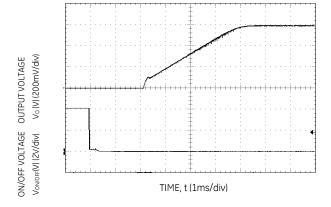
Figure 5. Typical Start-up Using On/Off Voltage ( $I_0 = I_{o,max}$ ).
