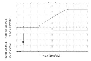
Figure 6. Typical Start-up Using Input Voltage ( $V_{IN} = 5V$ ,  $I_0 = I_{0,max}$ ).
