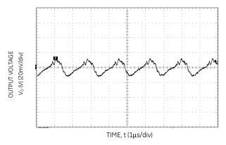
Figure 27. Typical output ripple and noise ( $V_{IN} = 5V$ ,  $I_0 = I_{O,max}$ ).
