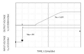
Figure 12. Typical Start-up Using Input Voltage ( $V_{IN} = 5V$ ,  $I_0 = I_{0,max}$ ).
