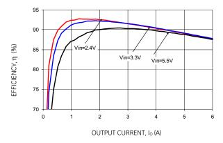
Figure 13. Converter Efficiency versus Output Current.
