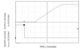
Figure 29. Typical Start-up Using On/Off Voltage ( $I_0 = I_{o,max}$ ).
