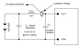
NOTE: Measure input reflected ripple current with a simulated source inductance ( $L_{\text{TEST}}$ ) of 1µH. Capacitor  $C_{\text{S}}$  offsets possible battery impedance. Measure current as shown above.
