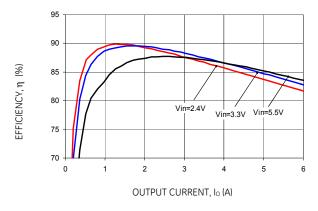
Figure 7. Converter Efficiency versus Output Current.
