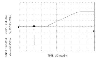
Figure 11. Typical Start-up Using On/Off Voltage ( $I_0 = I_{o,max}$ ).
