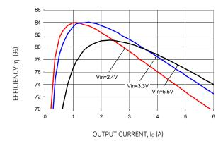
Figure 1. Converter Efficiency versus Output Current.
