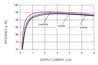
Figure 25. Converter Efficiency versus Output Current.
