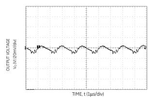
Figure 3. Typical output ripple and noise ( $V_{IN} = 5V$ ,  $I_0 = I_{O,max}$ ).
