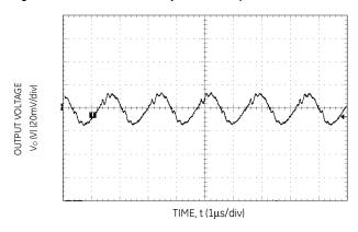
Figure 21. Typical output ripple and noise ( $V_{IN} = 5V$ ,  $I_0 = I_{O,max}$ ).
