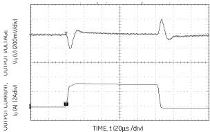
Figure 22. Transient Response to Dynamic Load Change from 0% to 50% to 0% with  $V_{\text{IN}}$ =5V.
