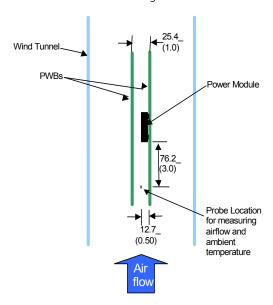
Figure 45. Thermal Test Setup.
