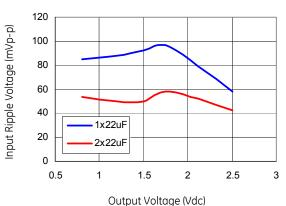
Figure 35. Input ripple voltage in mV, p-p for various output voltages with 1x22  $\mu$ F or 2x22  $\mu$ F ceramic capacitors at the input (6A load). Input voltage is 3.3V.
