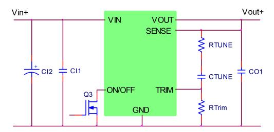
CIN1  $2 \times 22\mu\text{F}/6.3\text{V}$  ceramic capacitor CIN2  $47\mu\text{F}/6.3\text{V}$  bulk electrolytic
