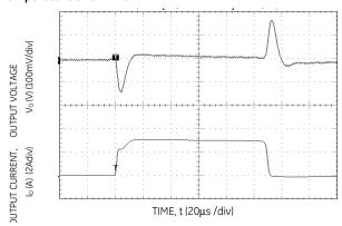
Figure 4. Transient Response to Dynamic Load Change from 0% to 50% to 0% with  $V_{\text{IN}=5\text{V}}$  .
