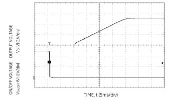
Figure 23. Typical Start-up Using On/Off Voltage ( $I_0 = I_{o,max}$ ).
