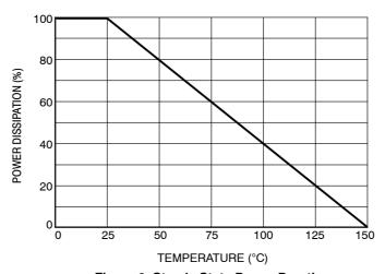
Figure 2. Steady State Power Derating
