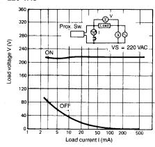
Note: When the current rating of the load is less than 10 mA, false operation may occur. This is normal, and the problem can be solved by installing a bleeder resistor in parallel with the load. Use the formulas given here to calculate the power rating and value of the resistor.
