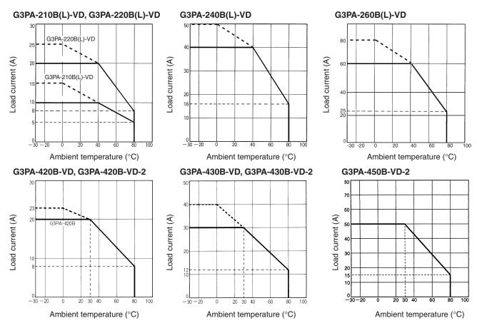
Note: Close mounting is possible for a maximum of three Units by reducing the load current by 20%. (A minimum clearance of 10 mm must be provided when mounting four or more Units.)
