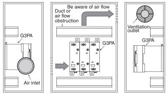
If the air inlet or air outlet has a filter, clean the filter regularly to prevent it from clogging and ensure an efficient flow of air.
