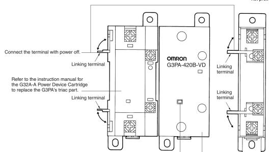
When the temperature indicator has turned from pink to red, the G32-A-A Power Device Cartridge may have malfunctioned, in which case the cartridge must be replaced with a new one.
