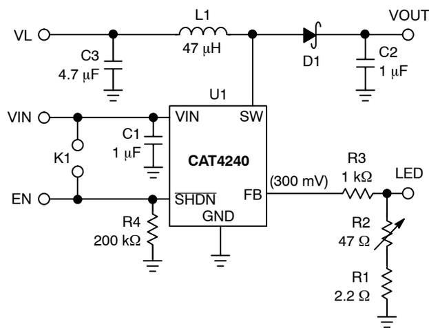
Figure 1. CAT4240AEVB Schematic
