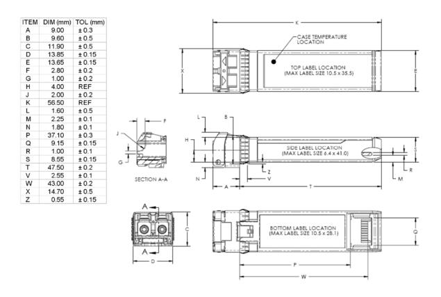
Figure 2. Mechanical Dimensions
