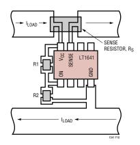
Figure 16. Recommended Layout for R1, R2 and R<sub>S</sub>
