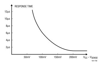
Figure 8. Response Time to Overcurrent
