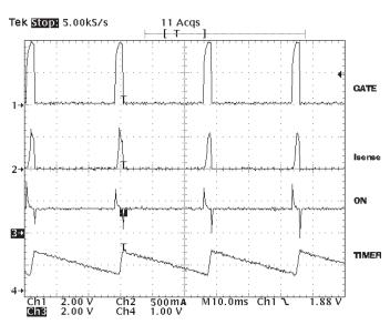
Figure 11. Automatic Restart Waveforms
