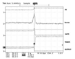
Figure 13. Overvoltage Waveforms
