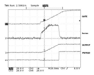
Figure 6. Power-Up Waveforms
