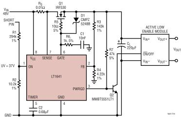
Figure 14. Active Low Enable Module
