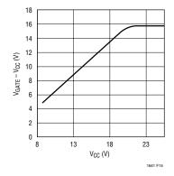
Figure 15. Gate Drive vs Supply Voltage
