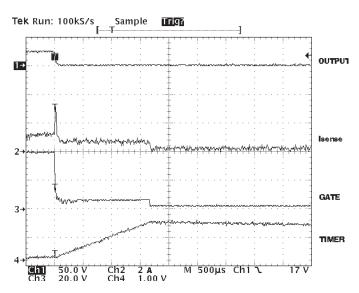
Figure 9. Short-Circuit Waveforms
