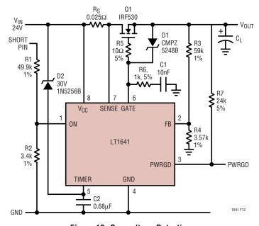
Figure 12. Overvoltage Detection
