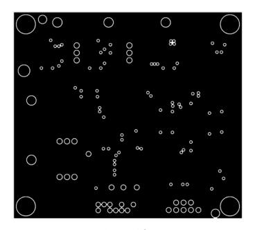
Figure 18. Layer 2 GND Plane
