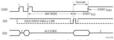
Figure 8. LTC2312-12 Entering/Exiting Nap Mode
