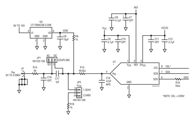
Figure 21. Partial 1563 Demo Board Schematic
