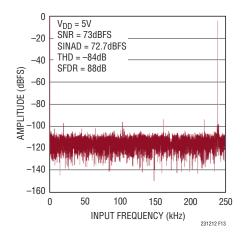
Figure 13. 16k Point FFT of the LTC2312-12 at  $f_{IN} = 259kHz$
