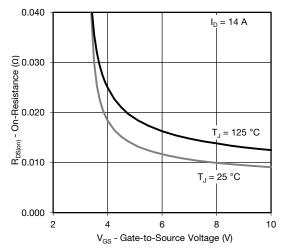
On-Resistance vs. Gate-to-Source Voltage
