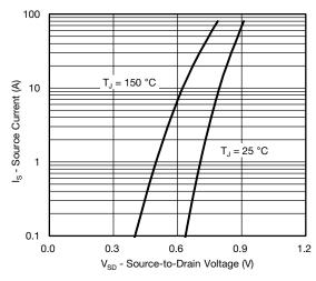
Source-Drain Diode Forward Voltage
