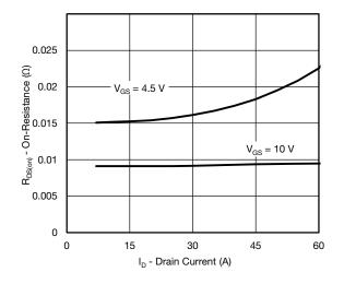
On-Resistance vs. Drain Current and Gate Voltage
