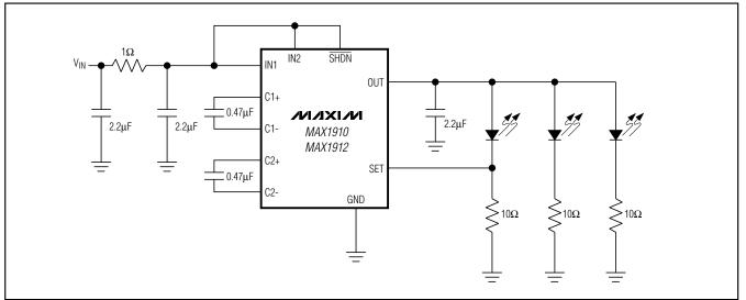
Figure 7. C-R-C Filter Reduces Ripple On the Input
