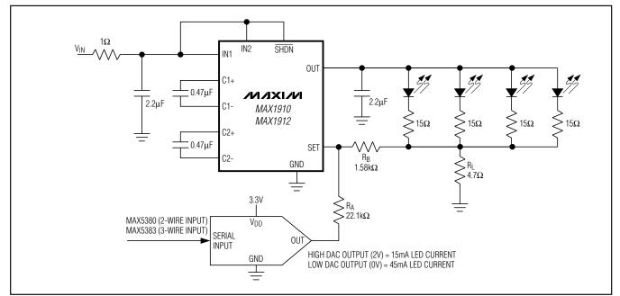
Figure 8. Circuit with SOT DAC for Intensity Control
