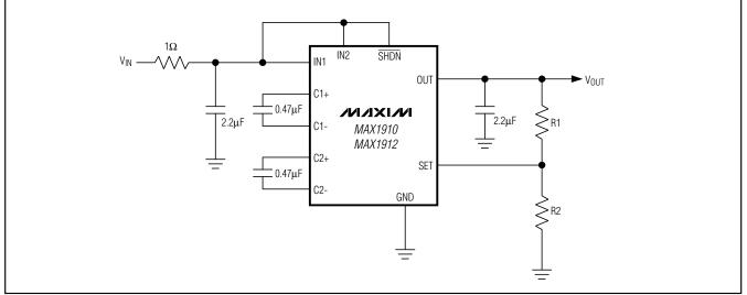
Figure 6. Output Voltage Set with a Resistor-Divider
