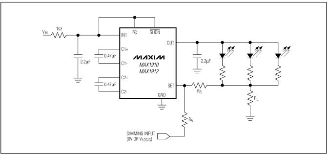
Figure 9. Using Digital Logic Input for Intensity Control
