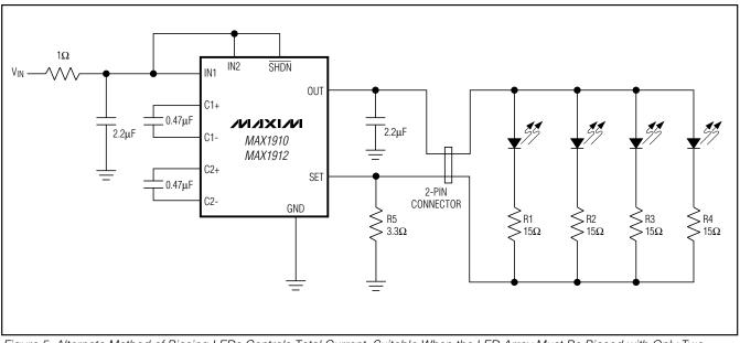
Figure 5. Alternate Method of Biasing LEDs Controls Total Current; Suitable When the LED Array Must Be Biased with Only Two Connections
