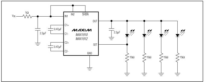
Figure 2. LED Biasing with the MAX1912
