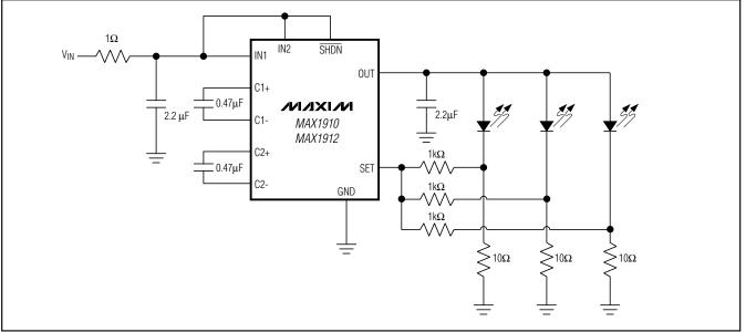
Figure 3. The MAX1912 Regulating Average Current Through LEDs
