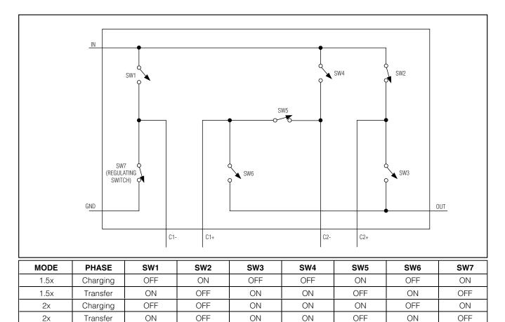
Figure 1. Functional Charge-Pump Switch Diagram (Switches Shown for 1.5x Charging Phase)
