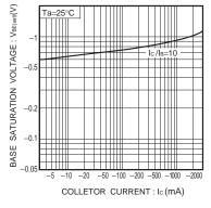
Fig.7 Base-emitter saturation voltage vs. collector current
