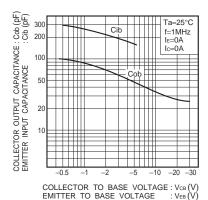
Fig.9 Collector output capacitance vs. collector-base voltage Emitter input capacitance vs.
