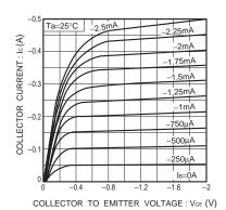
Fig.2 Grounded emitter output characteristics
