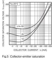
Fig.5 Collector-emitter saturation voltage vs. collector current (I)
