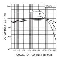
Fig.3 DC current gain vs. collector curren (I)
