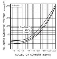
Fig.6 Collector-emitter saturation voltage vs. collector current (II)
