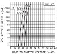
Fig.1 Grounded emitter propagation characteristics
