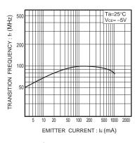
Fig.8 Gain bandwidth product vs. emitter current
