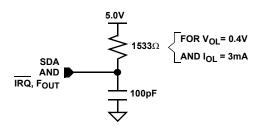
FIGURE 7. STANDARD OUTPUT LOAD FOR TESTING THE DEVICE WITH  $V_{\mathrm{DD}}$  = 5.0V
