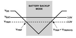
FIGURE 10. BATTERY SWITCHOVER WHEN VBAT > VTRIP
