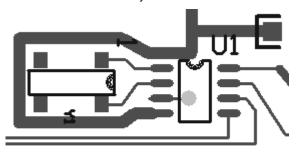
FIGURE 19. SUGGESTED LAYOUT FOR ISL1220 AND **CRYSTAL**
