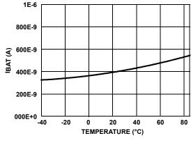
FIGURE 2. I<sub>BAT</sub> vs TEMPERATURE AT V<sub>BAT</sub> = 3V
