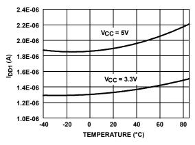
FIGURE 3. I<sub>DD1</sub> vs TEMPERATURE
