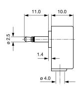
Cable diameter max. 4.0 mm
