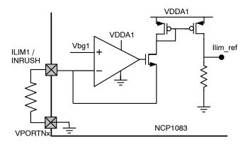
Figure 14. Current Limitation Configuration (Inrush & Ilim1 Pins)
