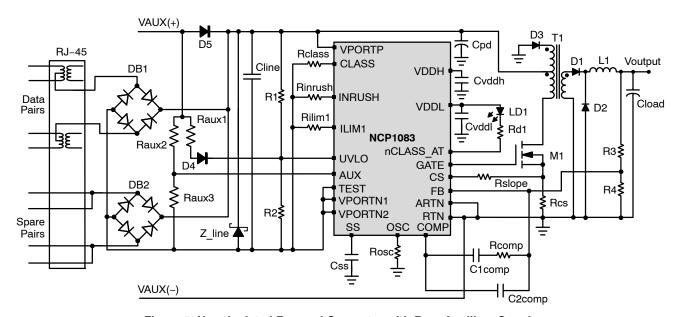
Figure 5. Non-Isolated Forward Converter with Rear Auxiliary Supply
