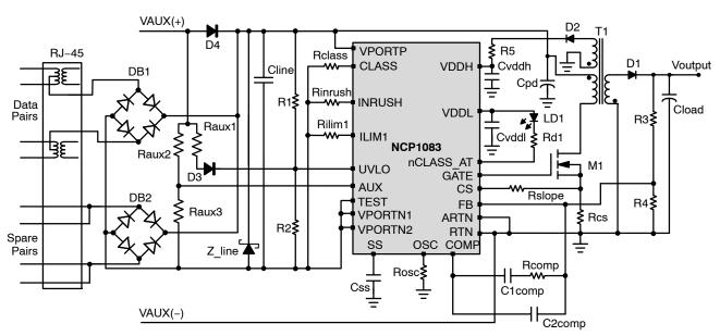
Figure 4. Non-Isolated Fly-back with Extra Winding and Rear Auxiliary Supply
