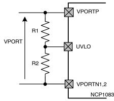
Figure 12. External UVLO Configuration
