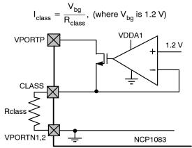
Figure 8. Classification Block Diagram
