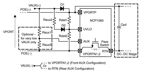
Figure 13. Front and Rear Auxiliary Supply Input with Support for Very Low Input Voltages
