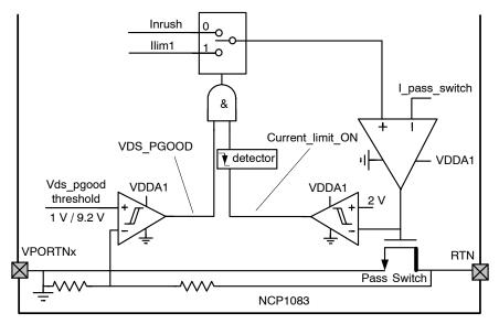
Figure 15. Inrush and Ilim1 Selection Mechanism
