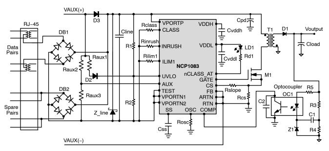
Figure 2. Isolated Fly-back Converter with Rear Auxiliary Supply
