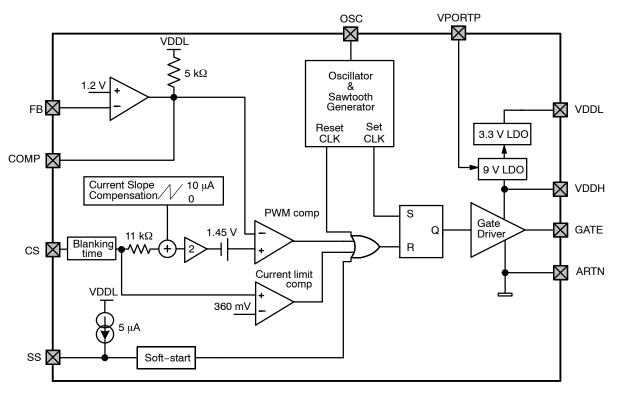
Figure 16. DC-DC Controller Block Diagram
