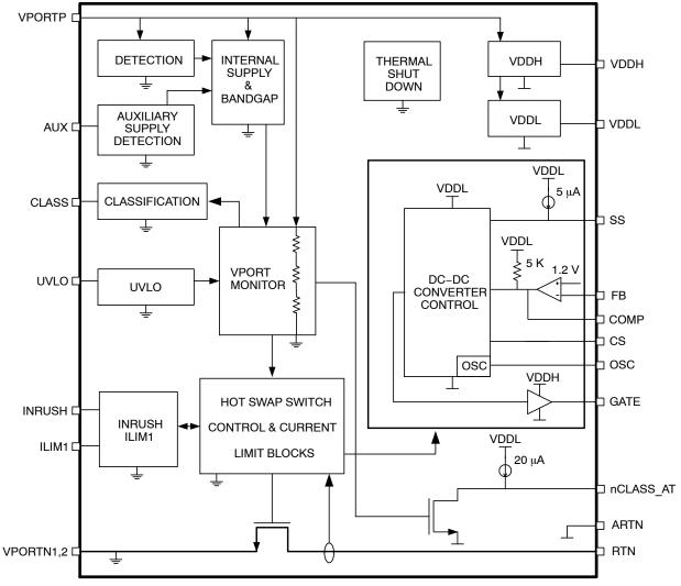
Figure 1. NCP1083 Block Diagram
