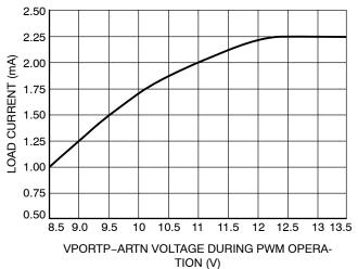
Figure 7. (Ivddh\_load+Ivddl\_load)max with Auxiliary Supply Operation
