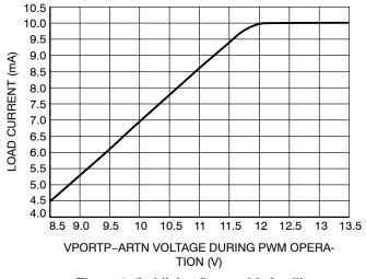
Figure 6. (Ivddl\_load)max with Auxiliary Supply Operation
