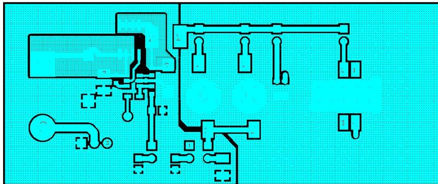
FIGURE 2: SP7601EB PC LAYOUT TOP SIDE
