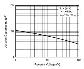
Fig. 5 - Typical Junction Capacitance
