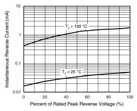
Fig. 4 - Typical Reverse Characteristics
