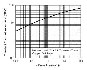
Fig. 6 - Typical Transient Thermal Impedance
