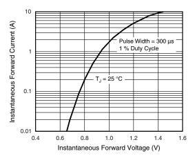
Fig. 3 - Typical Instantaneous Forward Characteristics
