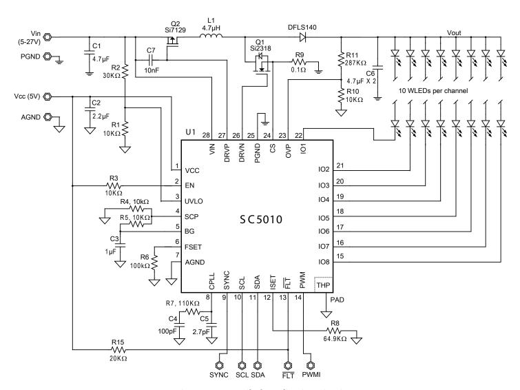
Figure 2 — Detailed Application Circuit
