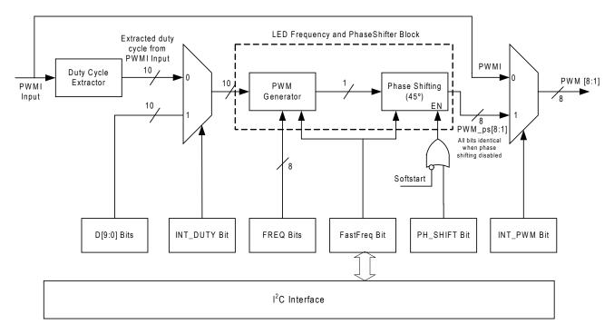
Figure 1— LED PWM Dimming Control
