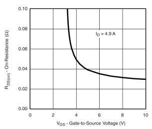
On-Resistance vs. Gate-to-Source Voltage
