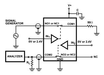
FIGURE 6. CROSSTALK TEST CIRCUIT
