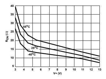
FIGURE 9. ON RESISTANCE vs SUPPLY VOLTAGE
