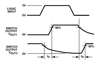
FIGURE 3A. MEASUREMENT POINTS (ISL84543 ONLY)
