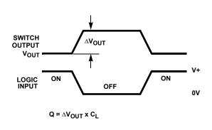
FIGURE 2A. MEASUREMENT POINTS
