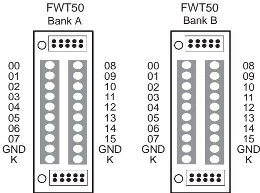
**Figure C-5. FWT50 Pinouts**
