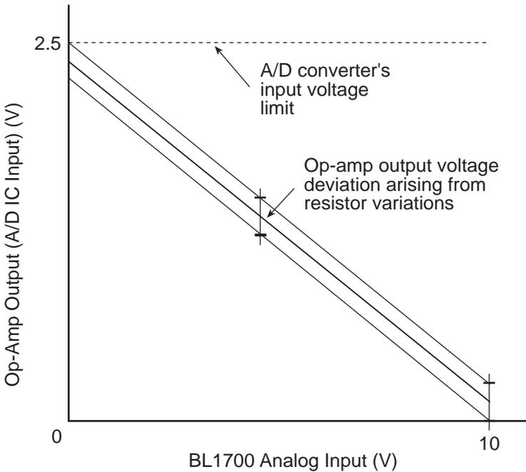
**Figure 3-9. Proper Input Range**
