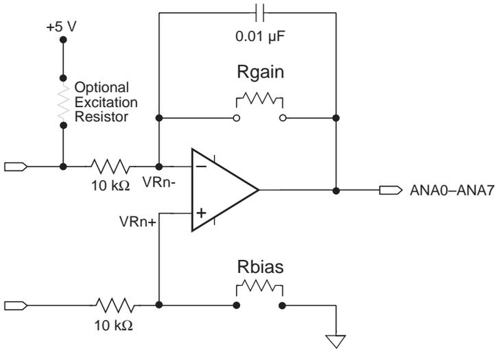
**Figure 3-7. Analog Conditioning Circuit**
