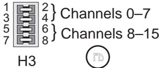
Figure D-2. Sinking Driver Jumper Configurations
