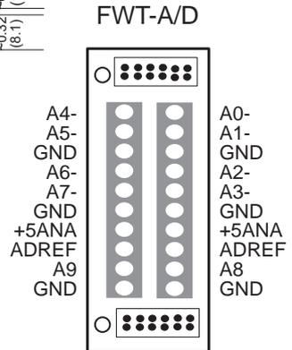
**Figure C-10. FWT-A/D Pinouts**
