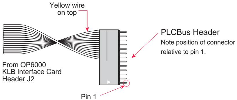
**Figure E-2. OP6000 Connection to PLCBus Port**
