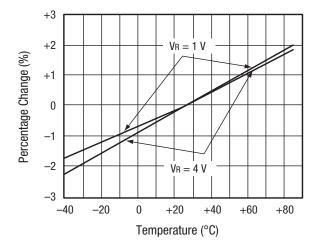
Figure 1. Relative Capacitance Change vs Temperature
