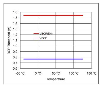
Figure 12: Brown-Out Protection Thresholds vs. Temperature
