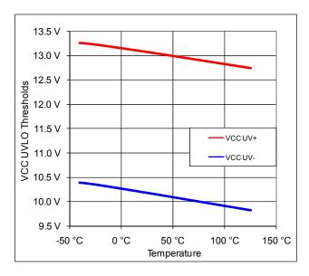
Figure 2: Undervoltage Lockout vs. Temperature
