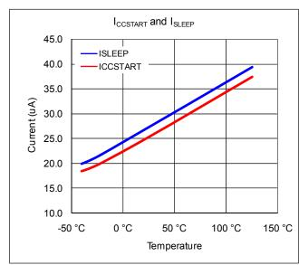
Figure 4: Startup Current and Sleep Current vs. Temperature
