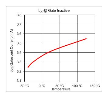
Figure 3: Icc Current vs. Temperature
