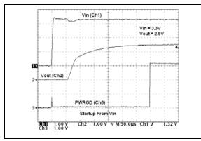
FIGURE 2-25: 2.5V (Adj.) Startup from V<sub>IN</sub>.
