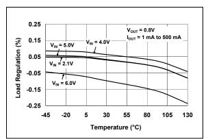
**FIGURE 2-17:** Load Regulation vs. Temperature (V<sub>OUT</sub> < 2.5V Fixed).
