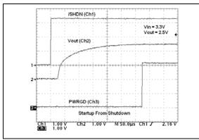
*FIGURE 2-26:* 2.5V (Adj.) Startup from Shutdown.
