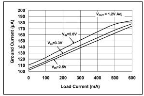
**FIGURE 2-2:** Ground Current vs. Load Current (Adjustable Version).
