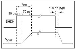
FIGURE 4-4: Shutdown Input Timing Diagram.
