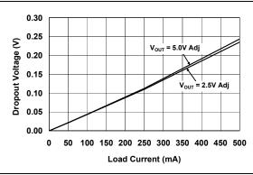
**FIGURE 2-7:** Dropout Voltage vs. Load Current (Adjustable Version).
