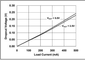
FIGURE 2-19: Dropout Voltage vs. Load Current.
