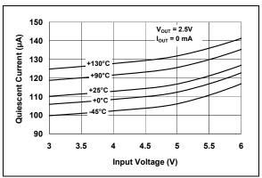
FIGURE 2-11: Quiescent Current vs. Input Voltage.
