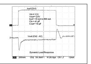
FIGURE 2-30: Dynamic Load Response (10 mA to 500 mA).
