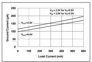
FIGURE 2-12: Ground Current vs. Load Current.
