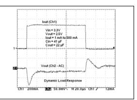
FIGURE 2-29: Dynamic Load Response (1 mA to 500 mA).
