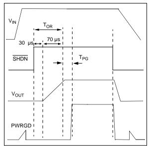
FIGURE 4-3: Power Good Timing from Shutdown.
