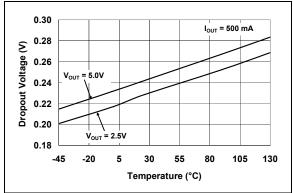
FIGURE 2-20: Dropout Voltage vs. Temperature.
