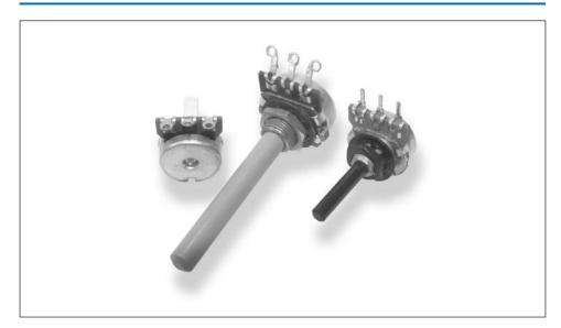
TE Connectivity will customize these neat 16mm diameter control potentiometers to suit your requirements. They comprise a printed carbon resistance element with 0.25 W current handling and are avaliable with various bush, termination and spindle styles.
